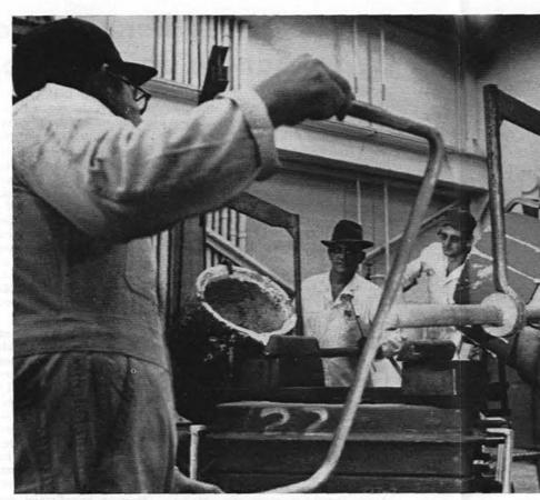
SMOOTH TEAM WORK is exhibited by Foundry- facility. Constant rate of flow into the mold is men during large pour. Inside the mold will form maintained up to 20 minutes until pour is coma 1000-lb. section of Sandia's new wind tunnel
